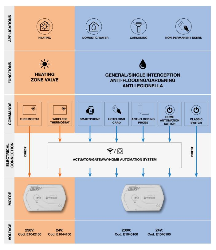
ON/OFF motor with auxiliary microswitch to manage the activation of the generator with the valve open.
