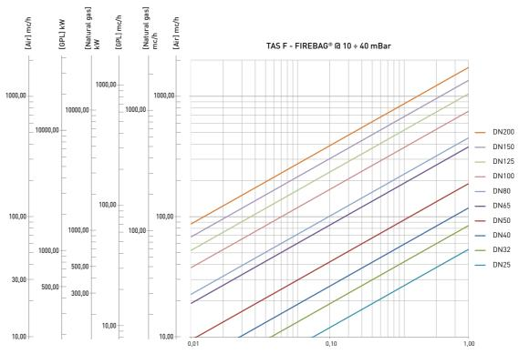
Gas Density [Natural gas] 0.717 kg/mc [GPL] 1.870 kg/mc Lower Heating Value [Natural gas] 35.88 mJ/mc [GPL] 85.32 mJ/mc
